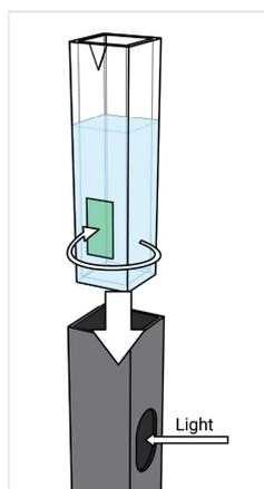
1. Turn the NanoCuvette™ 90 degrees such that the optical filter is not in the light path.
