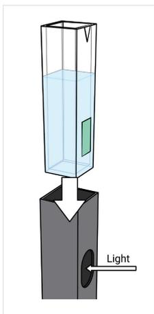
1. Carefully dispense DI-water into the NanoCuvette™.
