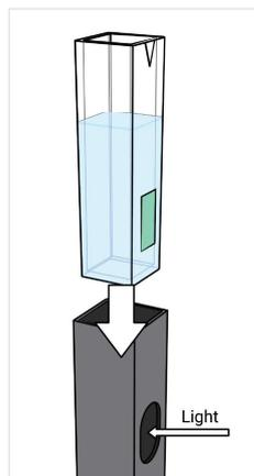
Follow the steps on the screen to measure the refractive index of your sample at the surface of the optical filter.
